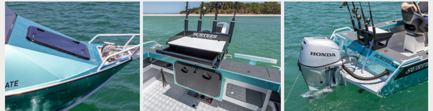
Large front hatch for easy access to anchor well and drum winch.
