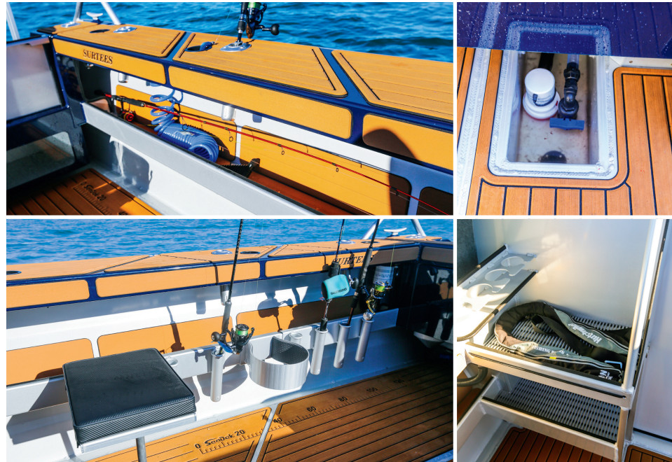
Clockwise from top: Shelving that runs the length of the cockpit makes great storage for rods, gaffs and the like; A centrally located sump houses the bilge pump; Provision has been made for a gas cooker in what is described as a 'mini-galley' located in front of the passenger seat; A feature of the boat is the Surtees clip-on rod and dive bottle holders and seat.
