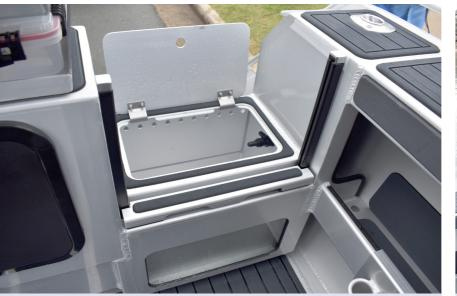
The live tank is cleverly located under the transom doorstep and the door itself slides up and down rather than inwards.
