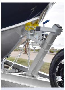
The trailer features a simple auto catch system for launching and retrieving, powered by gravity.
