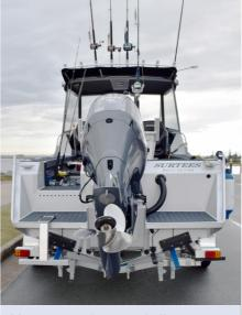
You can see the water ballast system at the apex of the transom. There's a cover that you can deploy to keep the water in there to soften the ride when conditions get rough.
