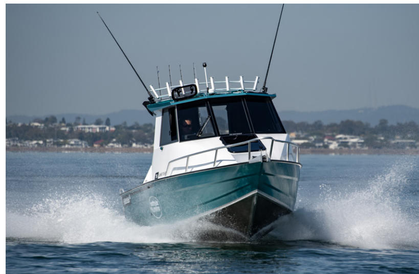
Left: You can see the spray chine doing their thing and deflecting water down and away from the hull. Right: Talk to Jason Comino at Northside Marine in Brisbane for more details about this beast of a rig.
